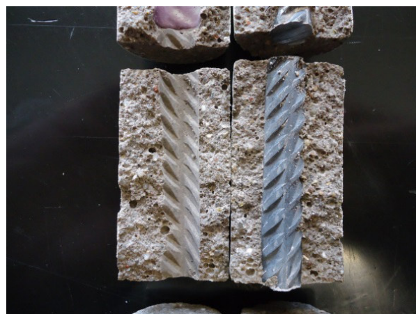
Fig.16: Split sample showing steel bar (right) and the rib-imprints in the mortar specimen (left).
